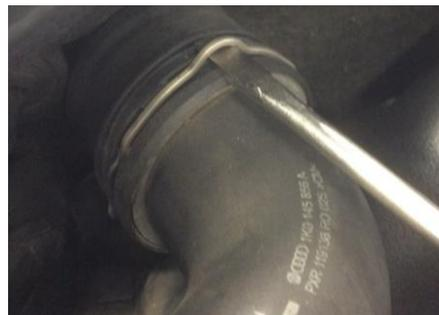
**D** Using tension clamp pliers slide the hose clamp back and remove the noise pipe from hose.
