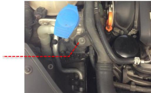
**C** Using a flat head screwdriver remove the noise pipe from the firewall coupling by prying the clip upward and removing from the plastic groove. Remove the coolant lines from the clamps on the side of the pipe.
