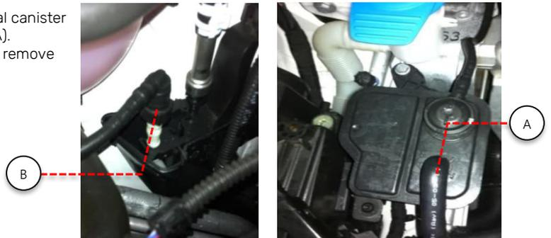
**B** Loosen the T30 bolt holding the noise pipe to the engine mount. The bolt is captive and will not remove from the bracket.
